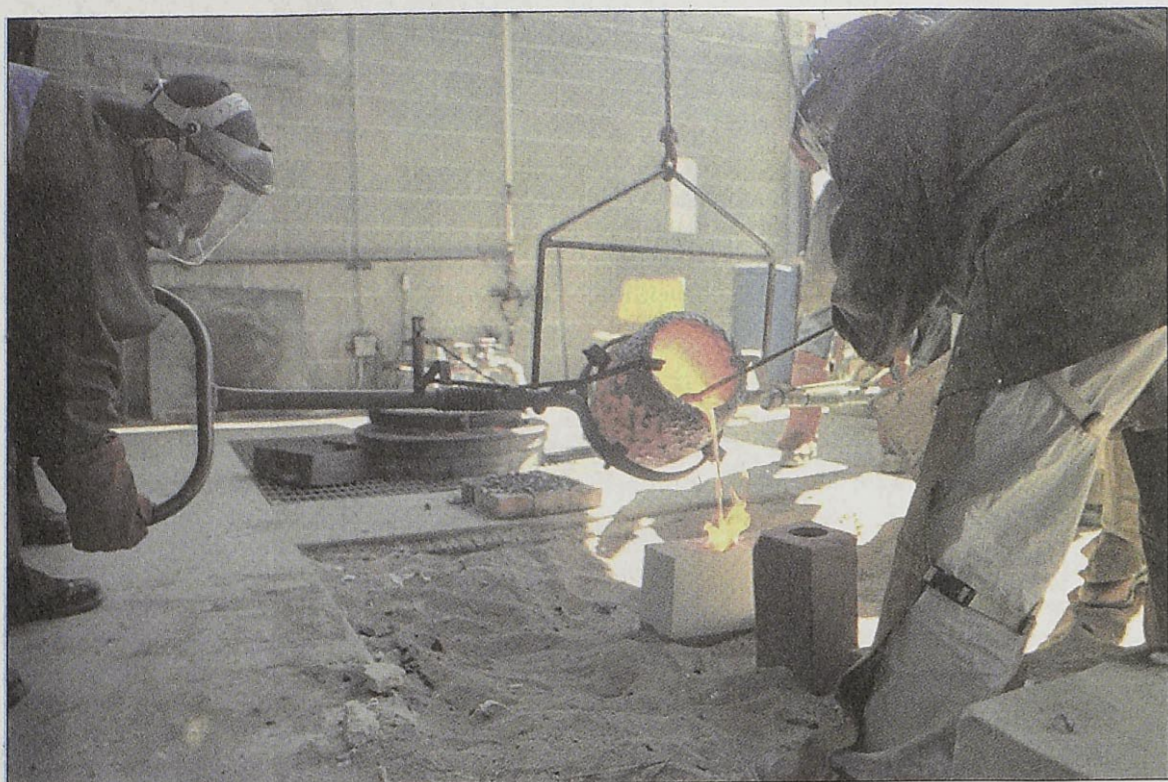
Student Darla Crask (left) uses crucible tongs to pour hot aluminum into molds, while alumni Amber Slater guides the team, giving students directions on where to position the crucible.
